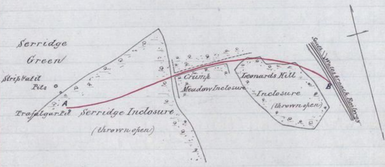
The Red line shews the branch applied for by Scale, CHAINS 20 to 1 Inch. M r . Corn s . Brain for the Trafalgar Colliery.
