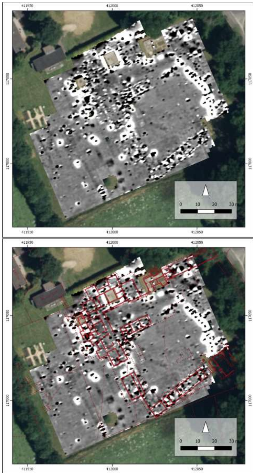
Figure 11: Destriped and interpolated results, greyscale from -10.0nT (white) to +10.0nT (black)
