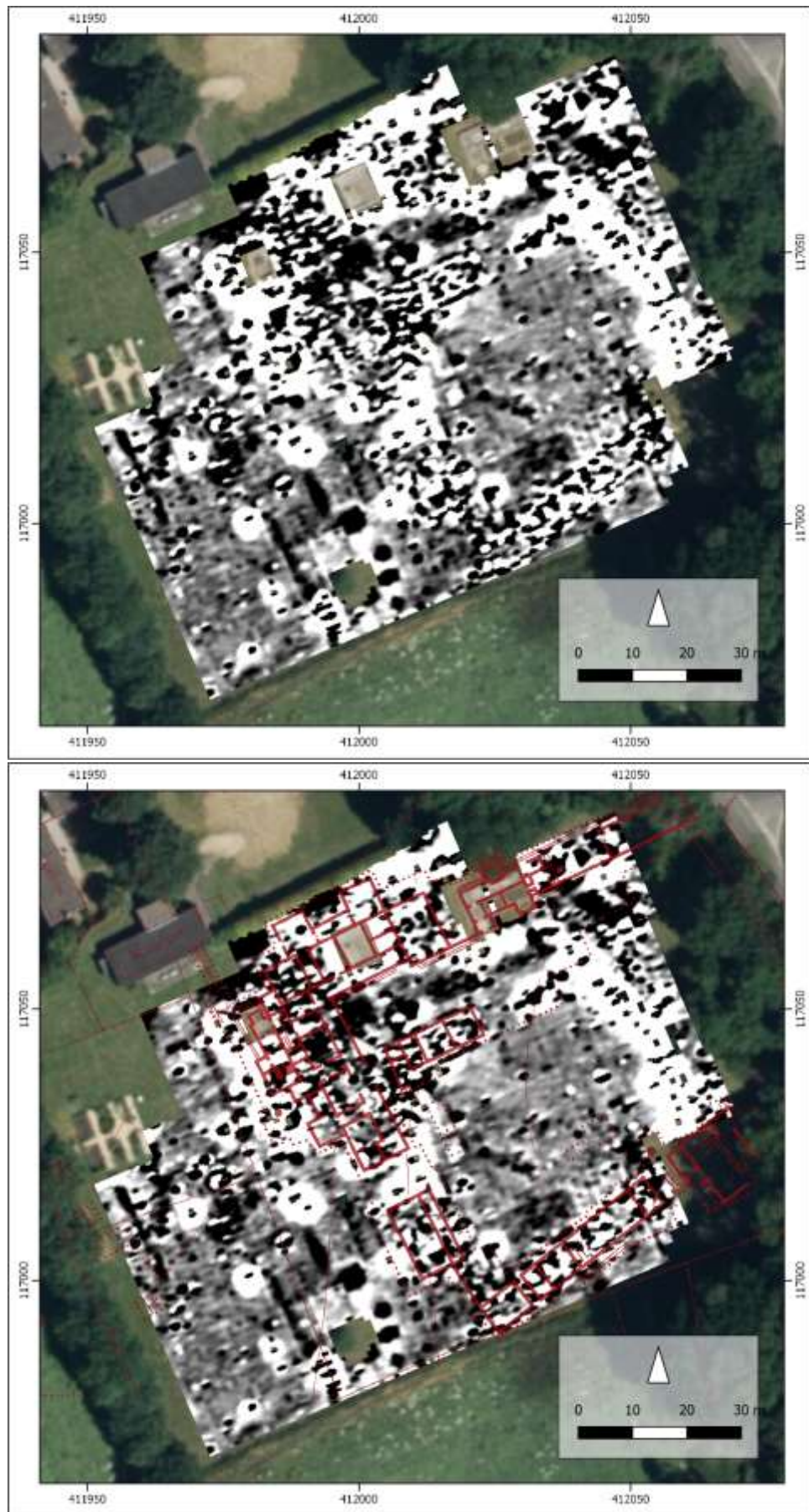
Figure 10: Destriped and interpolated results, greyscale from -2.0\text{nT} (white) to +2.0\text{nT} (black)
