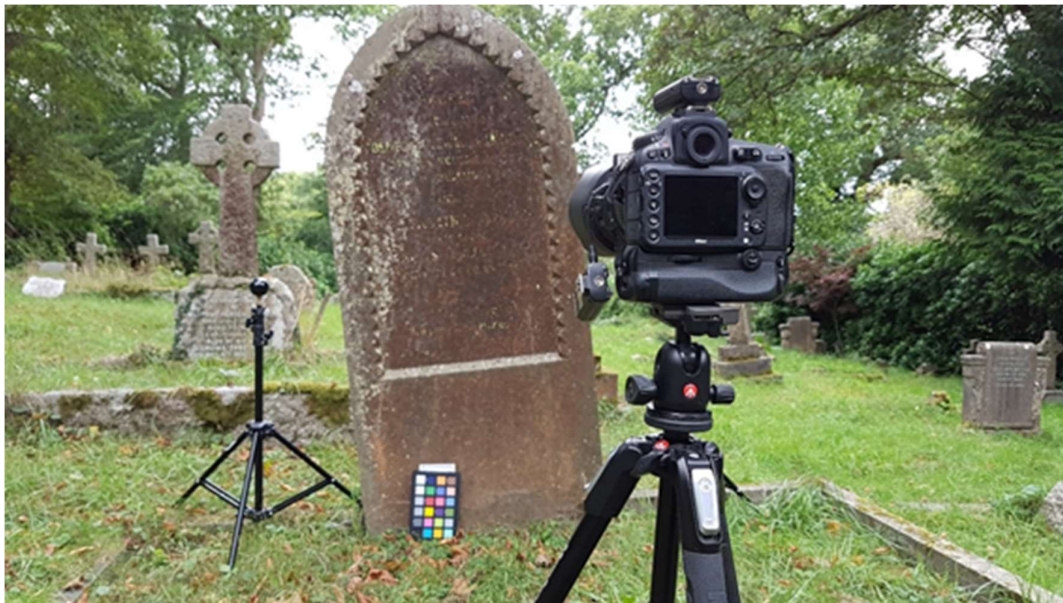
Highlight RTI setup capturing a gravestone at Burley, New Forest, UK. The camera and gravestone are in a stationary position, with the reflective ball found on the left-hand side, parallel to the gravestone. An external light source is then moved in a dome shape around the gravestone and successive images are captured. Photo by James
