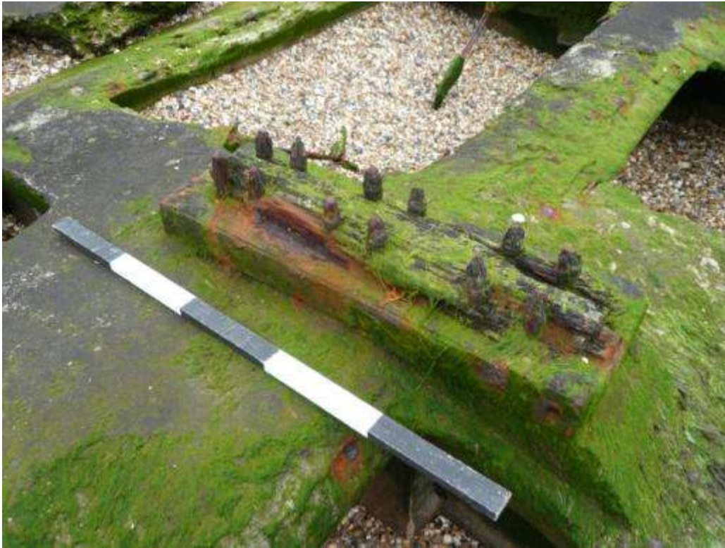
Figure 65 - Dorsal coupling bracket (with wood remnants)
