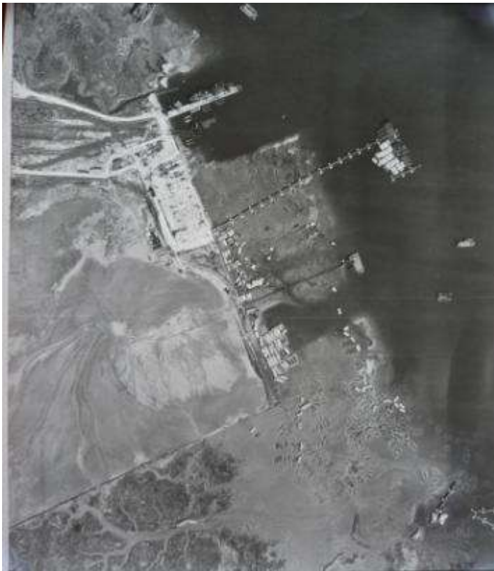
Figure 24 - EH12 Marchwood May 1947. Note the large number of Beetles at the end of the floating pier and other Mulberry Harbour remnants. Scale 1:5800
