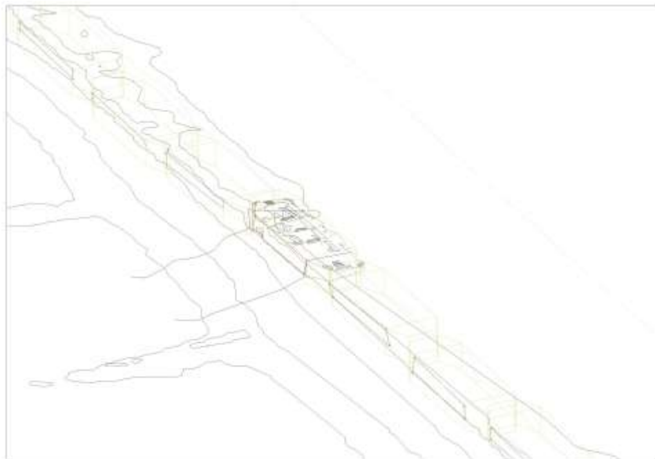
Figure 7 - Autocad depiction of Beetle no. 12 RTK points, combined with CCO LiDAR data. The degree of entrenchment in the bank is clear. The contour lines depict the beach slope at 50cm intervals, commencing at -0.5m below sea level (OD Newlyn)
