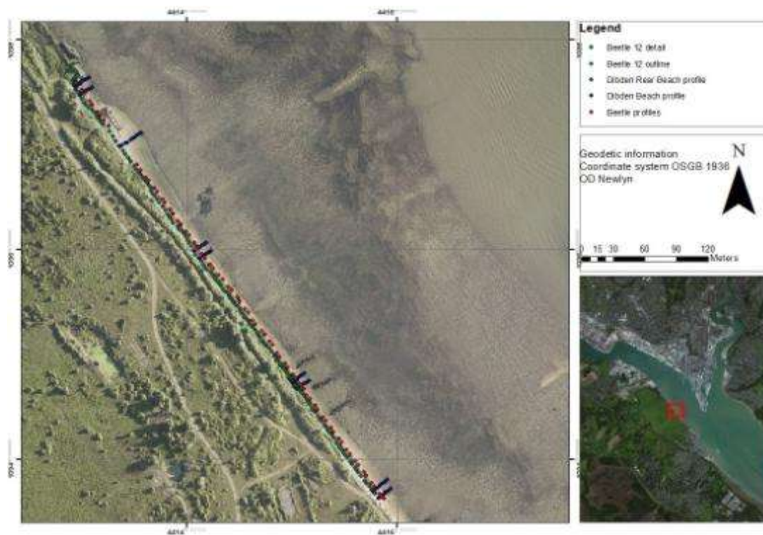
Figure 18 - Map showing the RTK Smartnet points taken in the course of the survey. Aerial photo courtesy of the CCO.
