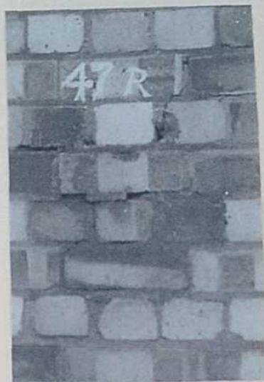
(b) Rear of wall showing cracks
